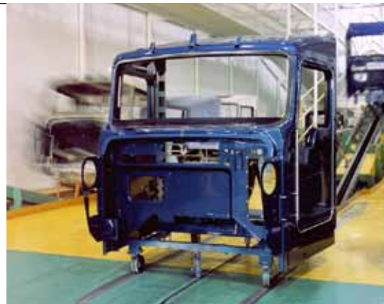
Coil-coated aluminum panels and a one-piece fiberglass roof, supported by an aircraft-grade aluminum alloy frame, produce a lightweight yet durable cab that is virtually immune to corrosion.
