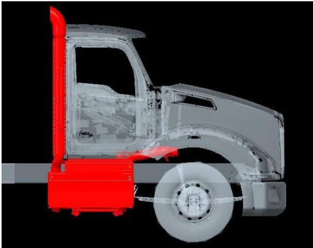
FIGURE 5-8. RHUC DPF/SCR SOC Tailpipe – RH View
