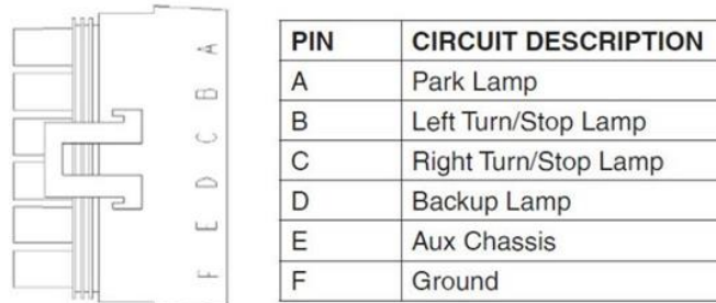
FIGURE 10-39. Mating Connector: Packard PN 12020789
