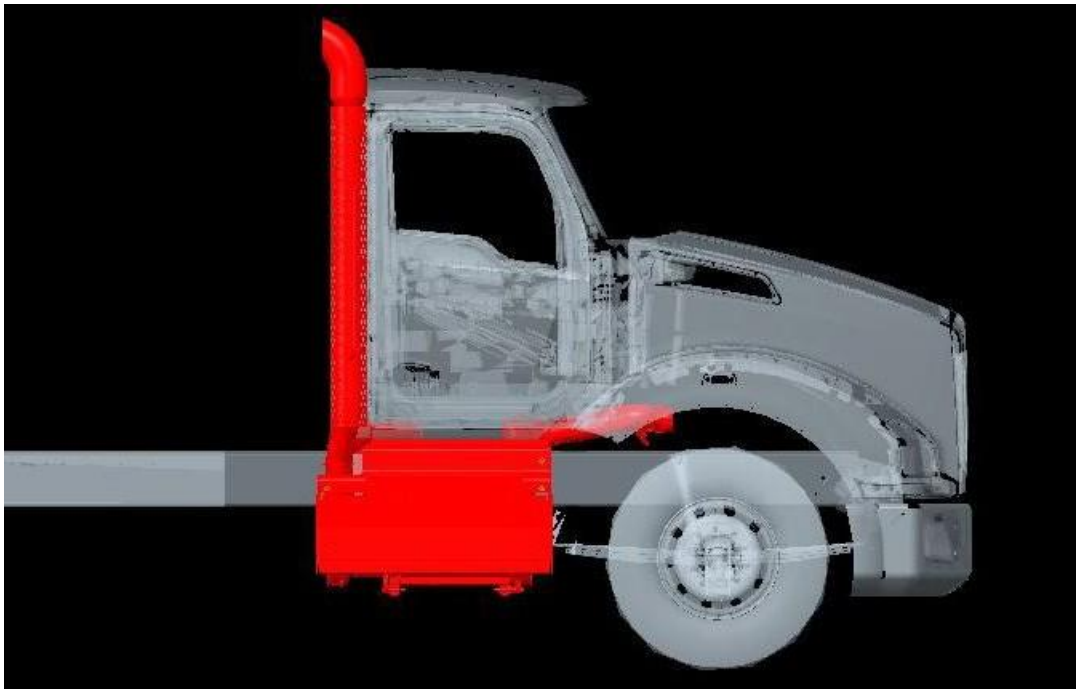
FIGURE 5-12. RHUC DPF/SCR Dual SOC Tailpipes – RH View
