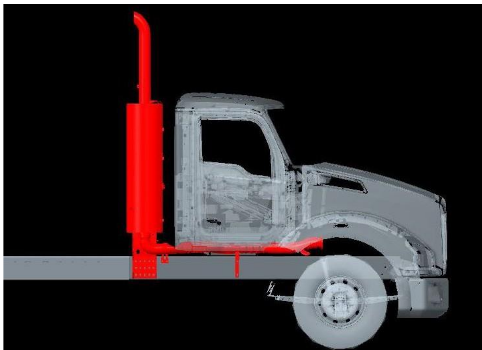
FIGURE 5-24. Independent BOC DPF/SCR w/BOC Tailpipe – RH View
