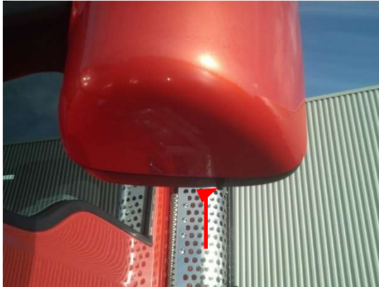
Figure 2-3 Aerodynamic Mirror OAT Sensor Location
