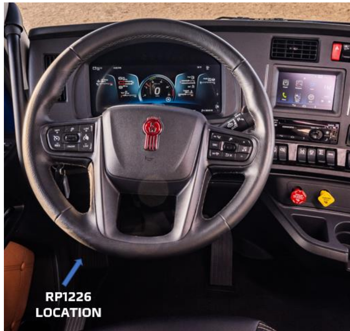
Figure 4-15. Standard RP1226 Location (Driver's Side Kick Panel)
