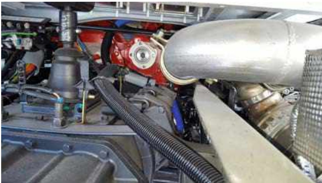
FIGURE 4-4. REPTO Flywheel Housing
