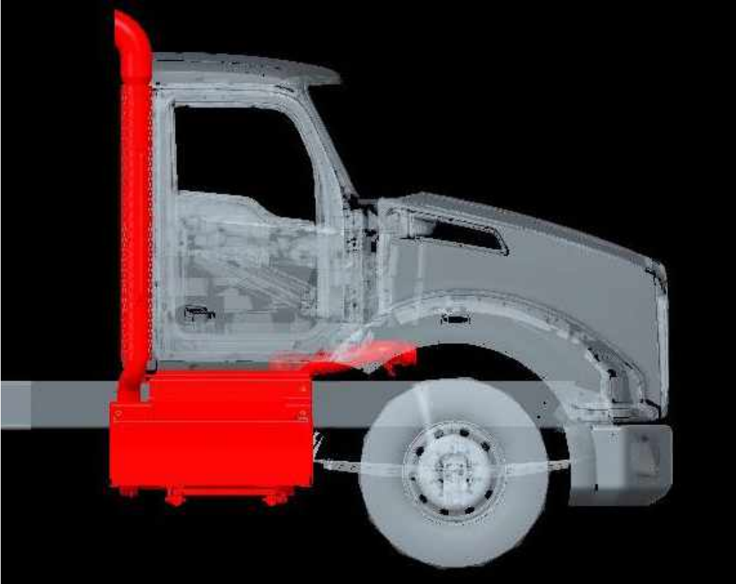
FIGURE 5-5. Right view of Right Hand Under DPF/SCR with Single Side of Cab Tailpipe
