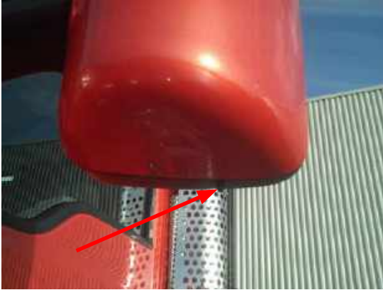
FIGURE 2-3: Aerodynamic Mirror OAT Sensor Location
