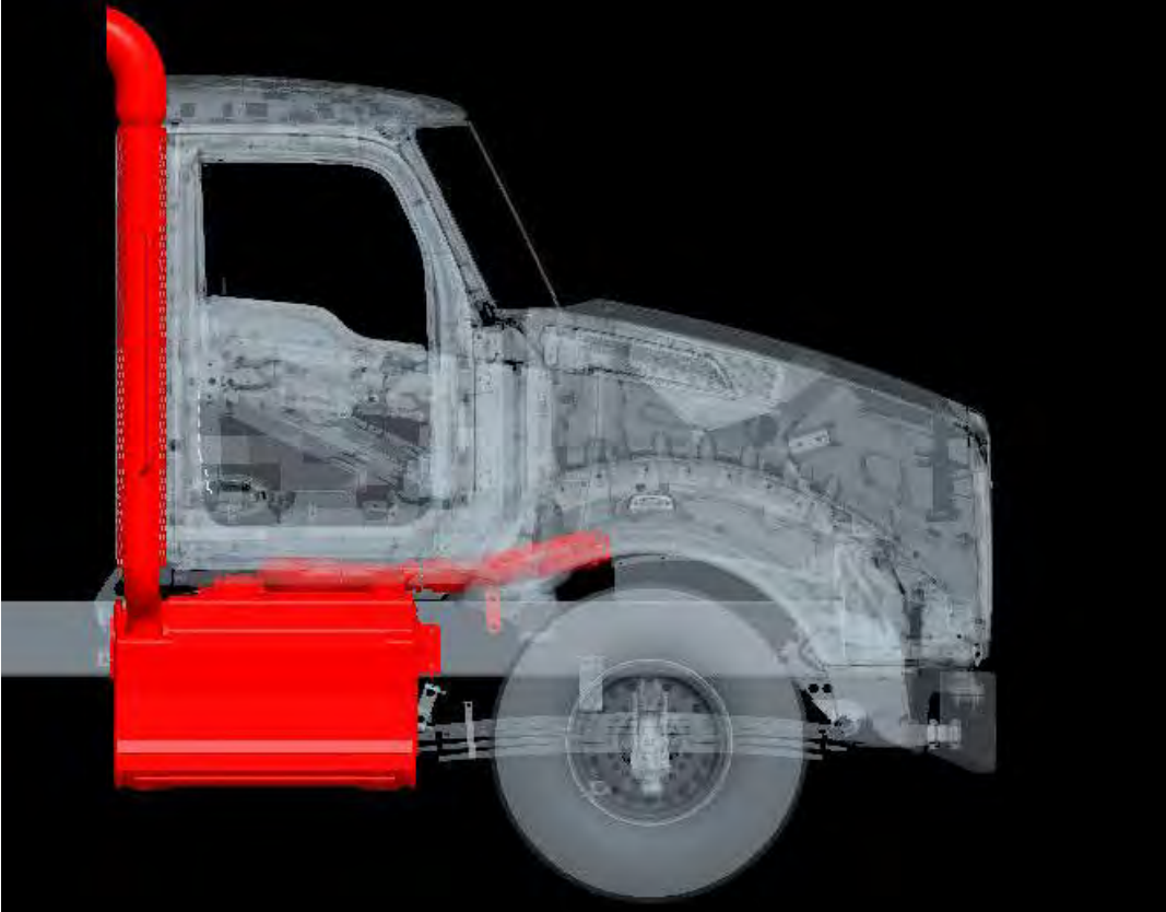
FIGURE 5-11: Right view of Right Hand Under DPF/SCR with Single Side of Cab Tailpipe
