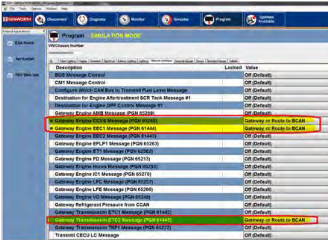
FIGURE 4-33. Remote PTO Control over BCAN with PTO ON/OFF Switch Signal over BCAN – ESA Settings for T680/T880
