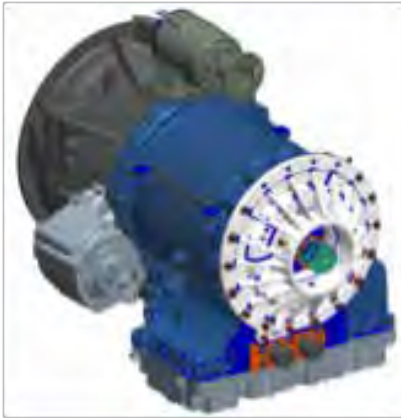
FIGURE 4-4. Allison 4000 Series Transmission PTO Locations
