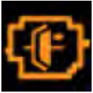
FIGURE 4-19. Rear Axle Declutch Telltale
