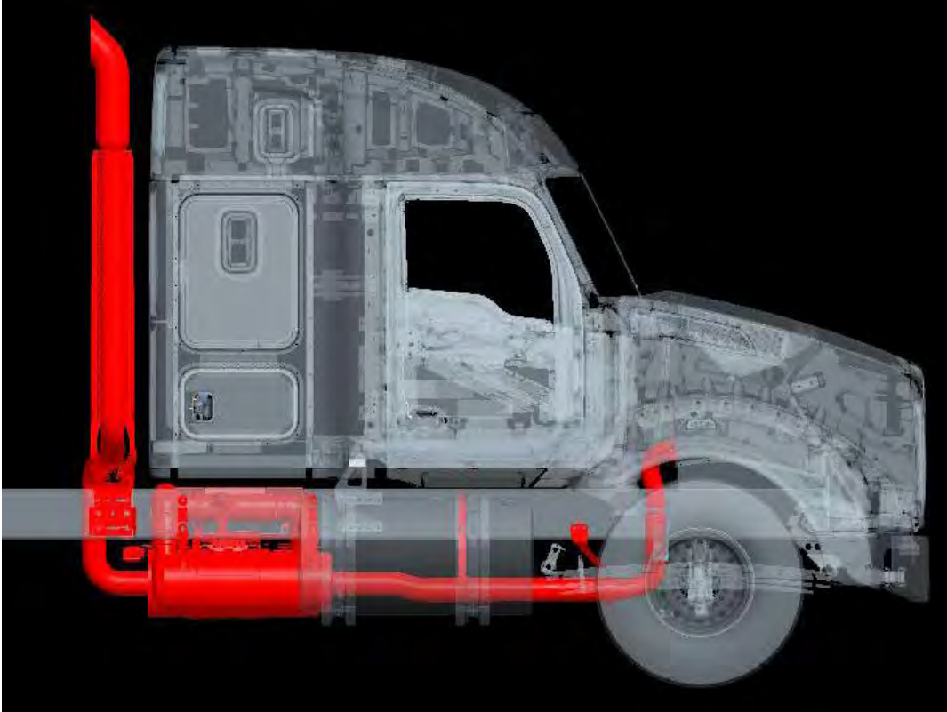
FIGURE 5-51: Right View of Horizontal Crossover DPF/SCR with Single Back of Sleeper Tailpipe (52" Sleeper)
