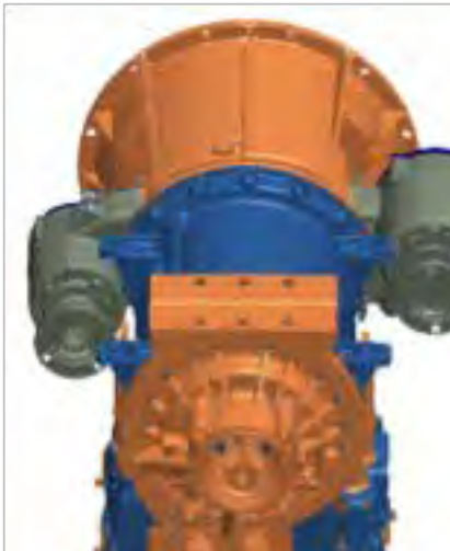
FIGURE 4-5. Allison 3000 Series Transmission PTO Locations
