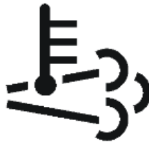
Figure 5.1 – HEST Warning Light
