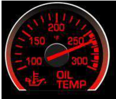
Figure 76: Oil Temp Gauge in warning state
