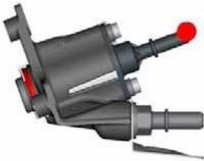
Figure 4-3 Measurement Location of DEF Dosing Module (Injector)
