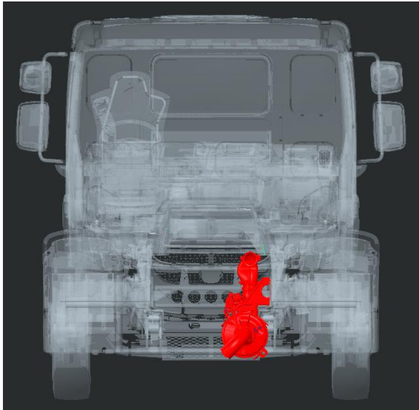
Figure 4-6.4 Back view of Horizontal Exhaust Canister with Horizontal Tailpipe
