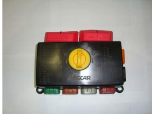
Figure 7.6.1 Pwer Distribution Center
