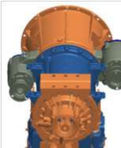
FIGURE 4-5. Allison 3000 Series Transmission PTO Locations
