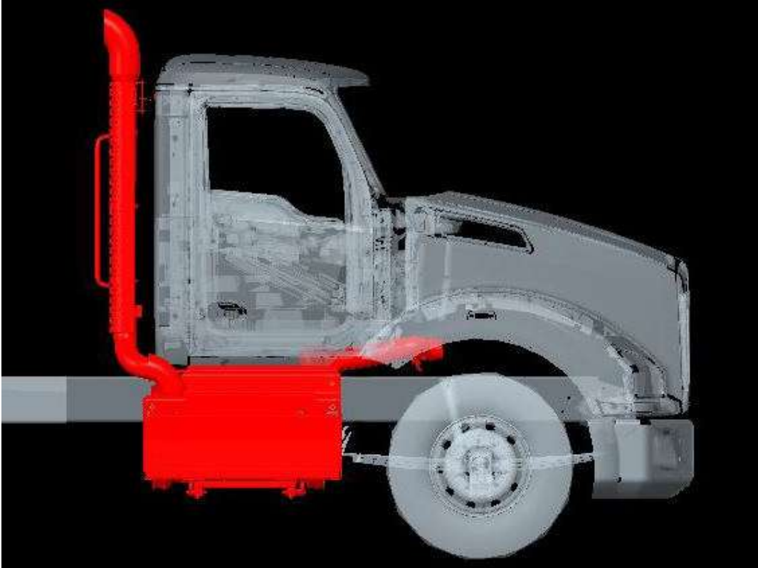
FIGURE 5-13. Right View of Right Hand Under DPF/SCR with Single Back of Cab Tailpipe
