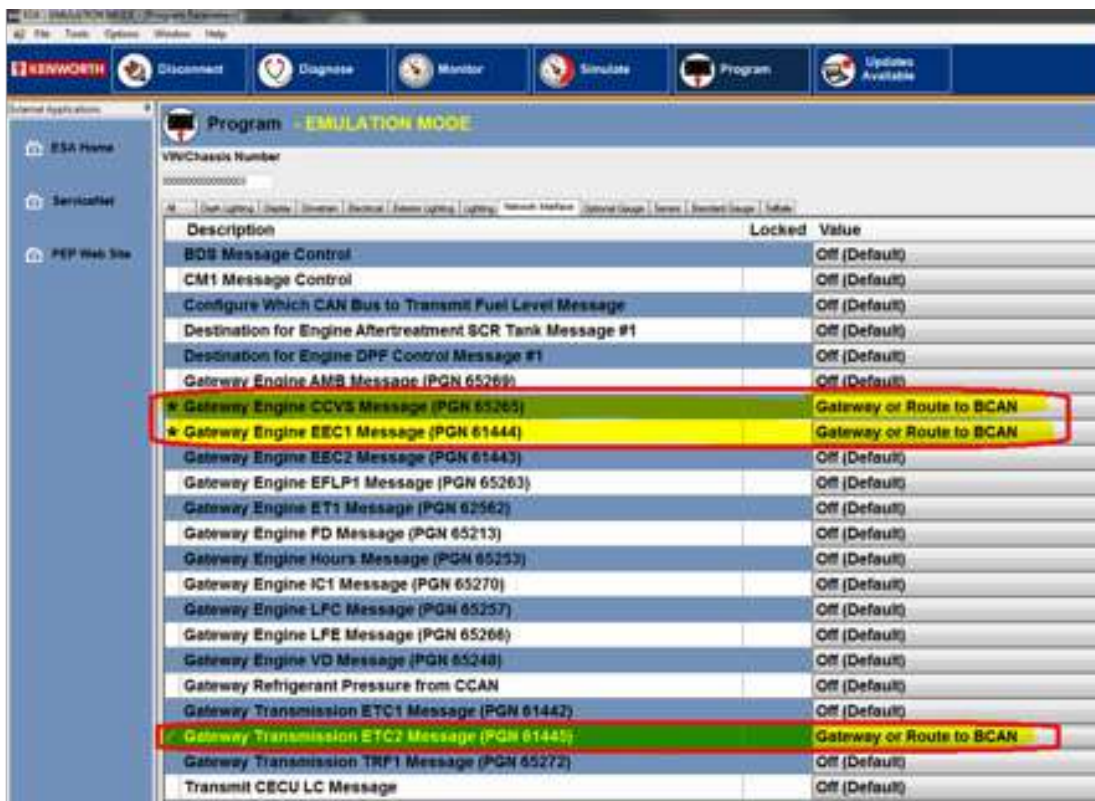
FIGURE 4-36. Remote PTO Control over BCAN with PTO ON/OFF Switch Signal over BCAN – ESA Settings for T680/T880
